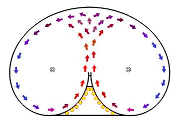
At the centre of each flow pattern is an "eye" in the circulation path as marked with double circles in the diagram above.
