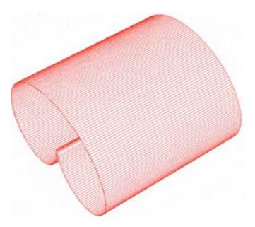
Heating the lower part of the tank and bubbling gas from along the central cusp inside the tank causes the liquid contents to rise vertically from the centreline of the tank and then to form two opposing circulation patterns, being constrained by the minimum energy curve of the tank walls. This results in very efficient and thorough mixing of the contents which ensures complete degradation of the organic matter and the maximum production of methane:
